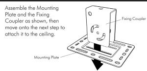
NOTE If mounting onto an analed ceiling, ensure the Fixing Coupler is in the correct orientation.
