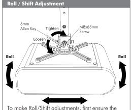
weight of the projector is supported. Then loosen the M8x65mm Screw with the supplied 6mm Allen Key, and adjust to your desired position. Re-tighten the screw firmly.
