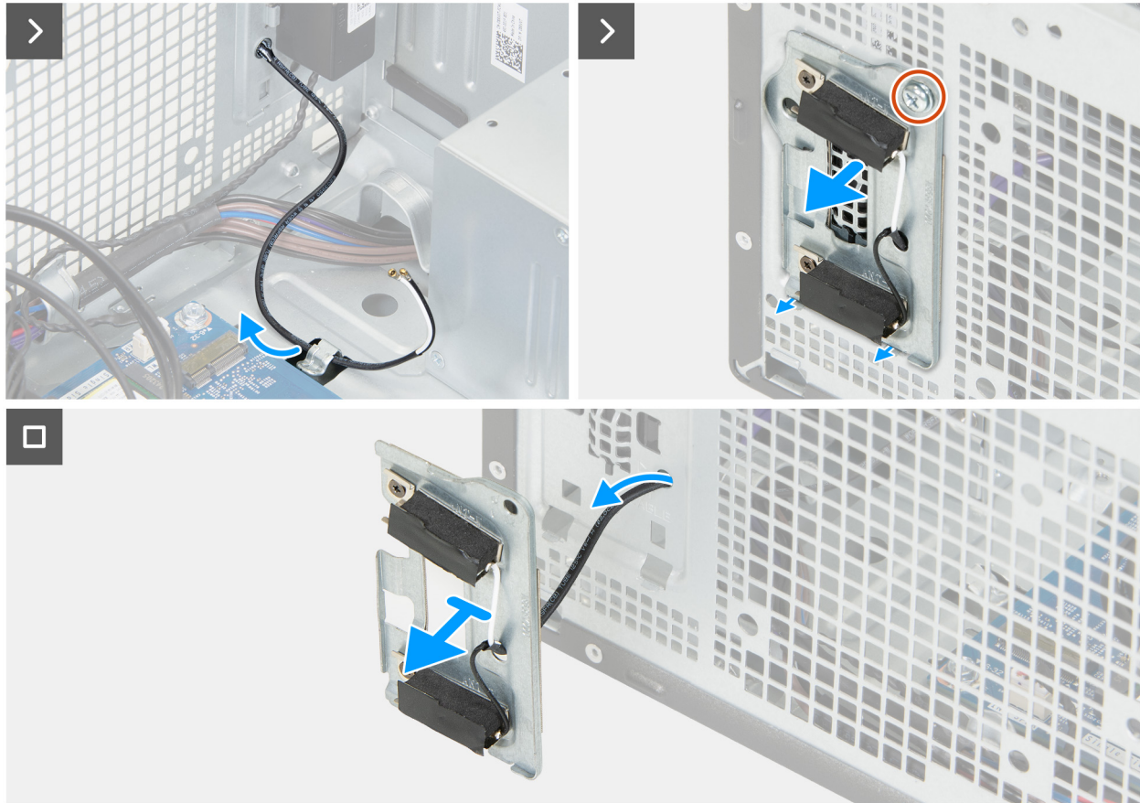
Figure 60. Removing the antenna modules
