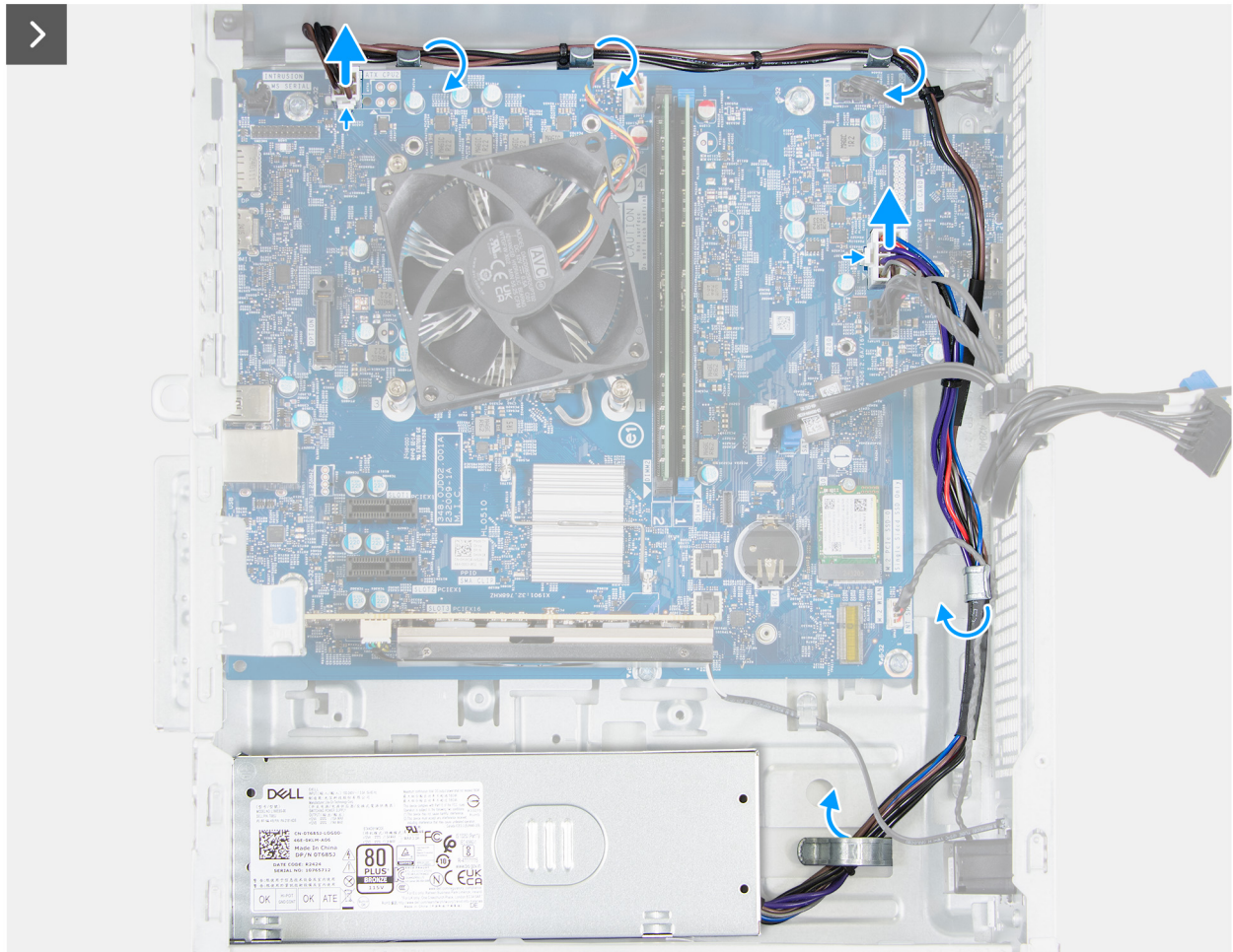
Figure 62. Removing the power-supply unit
