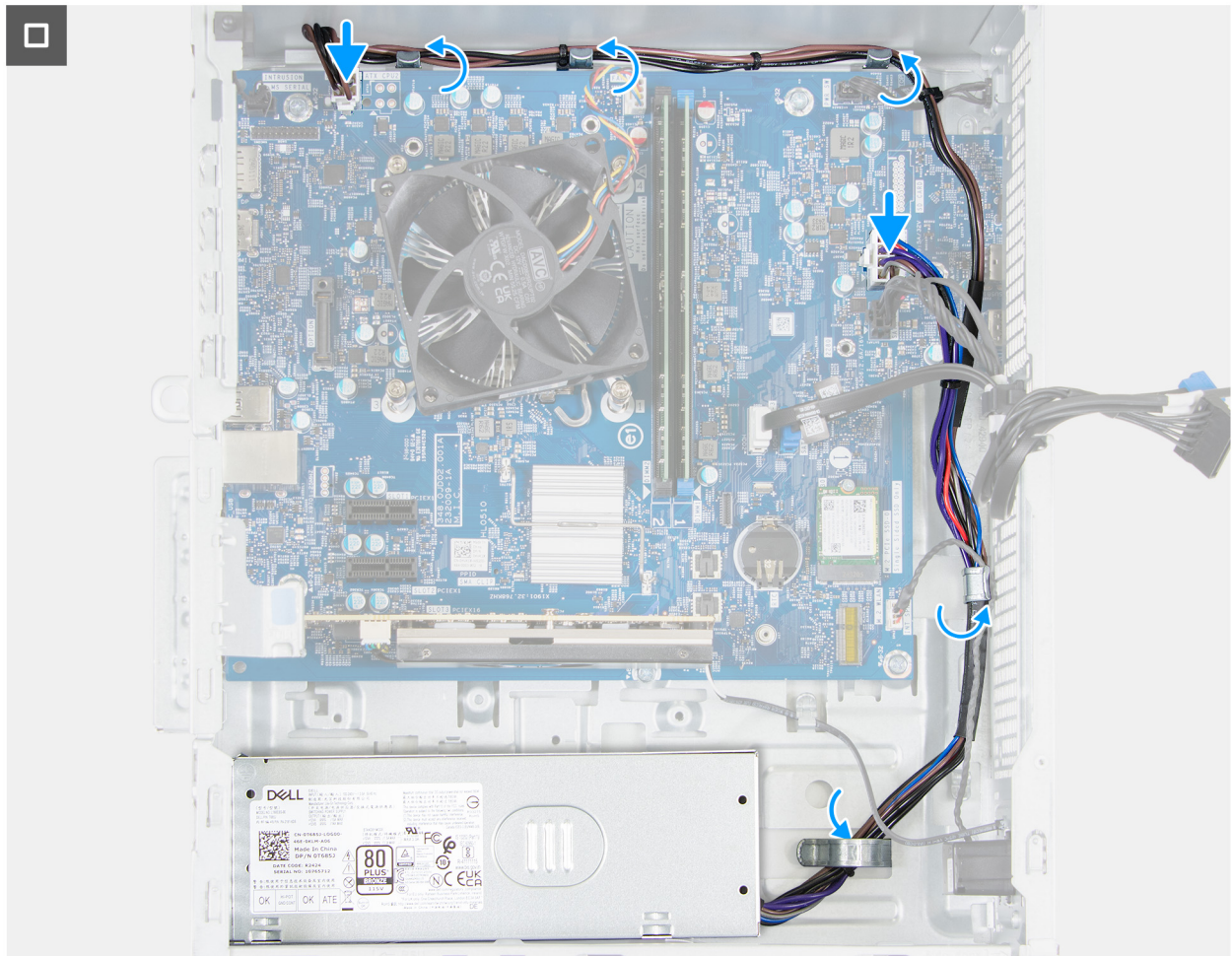
Figure 65. Installing the power-supply unit
