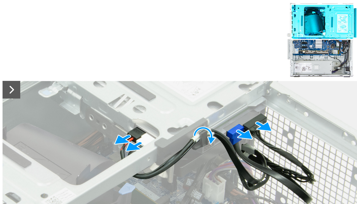
Figure 42. Removing the drive bay
