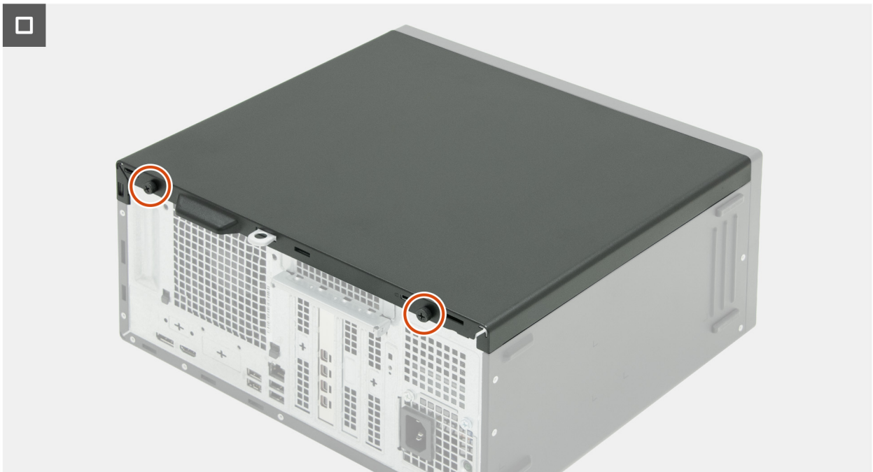
Figure 16. Installing the left-side cover
