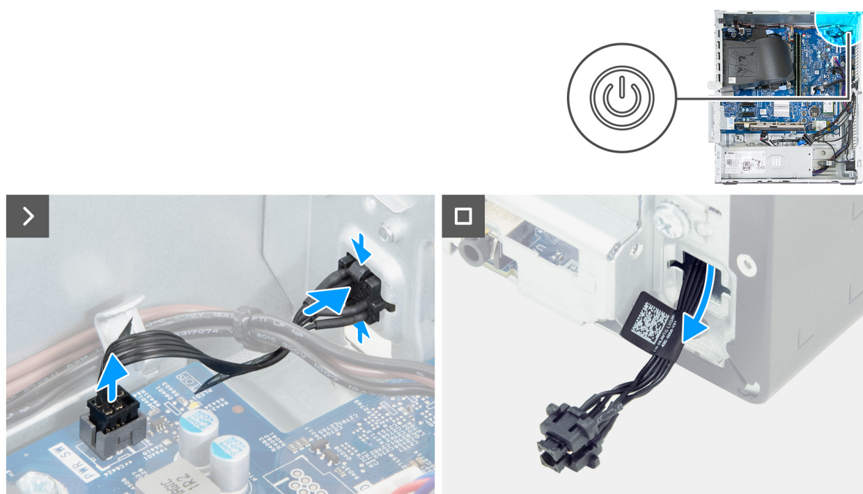
Figure 50. Removing the power button
