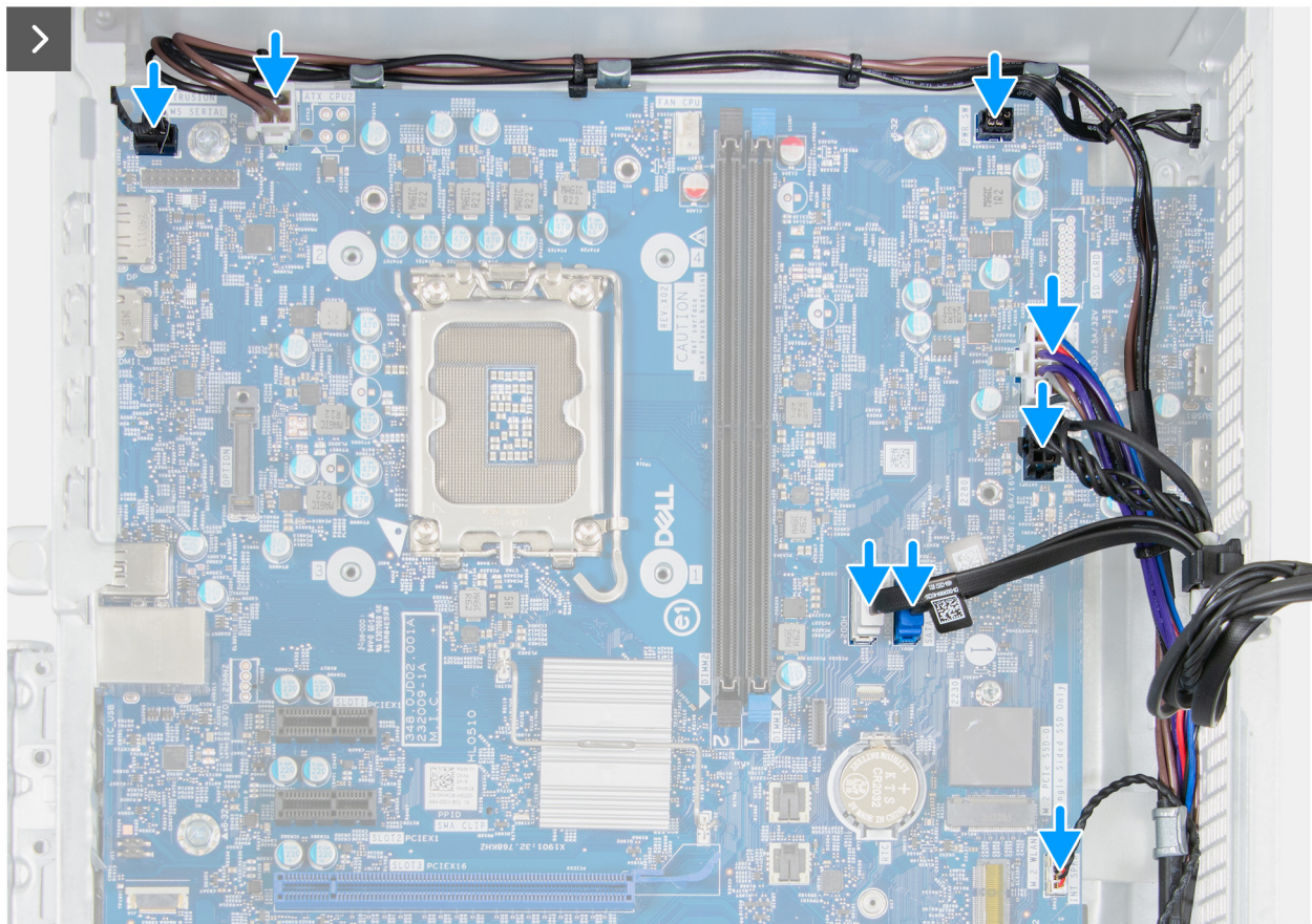
Figure 78. Installing the system board
