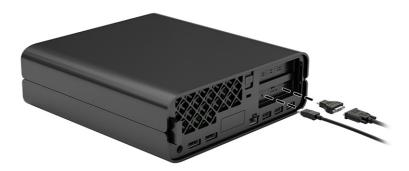
Connect the other ends of the monitor cables to the monitors.
