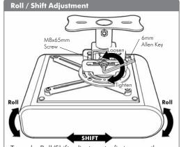
To make Roll/Shift adjustments, first ensure the weight of the projector is supported. Then loosen the M8x65mm Screw with the supplied 6mm Allen Key, and adjust to your desired position. Re-tighten the screw firmly.
