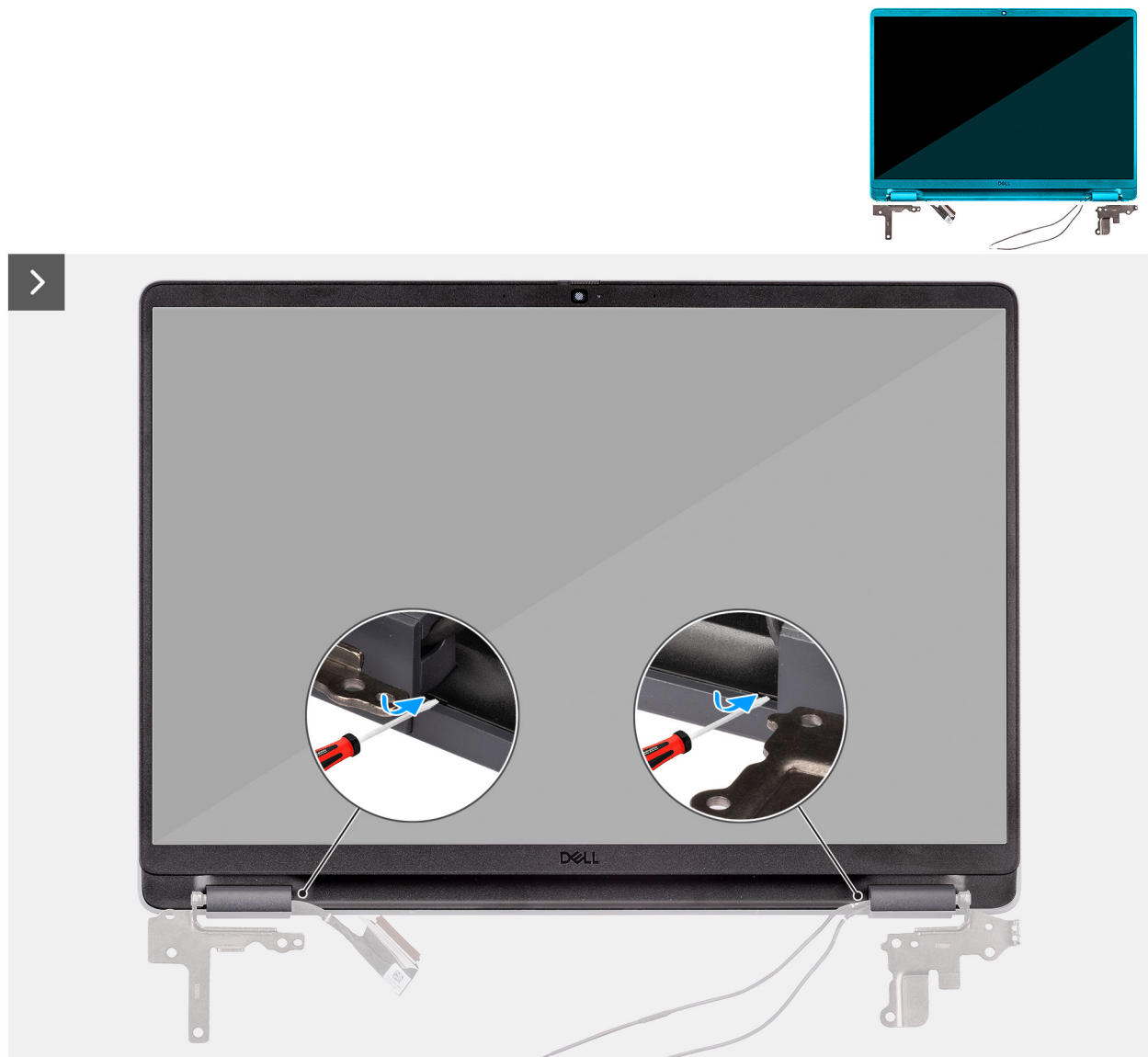
Figure 67. Removing the display bezel
