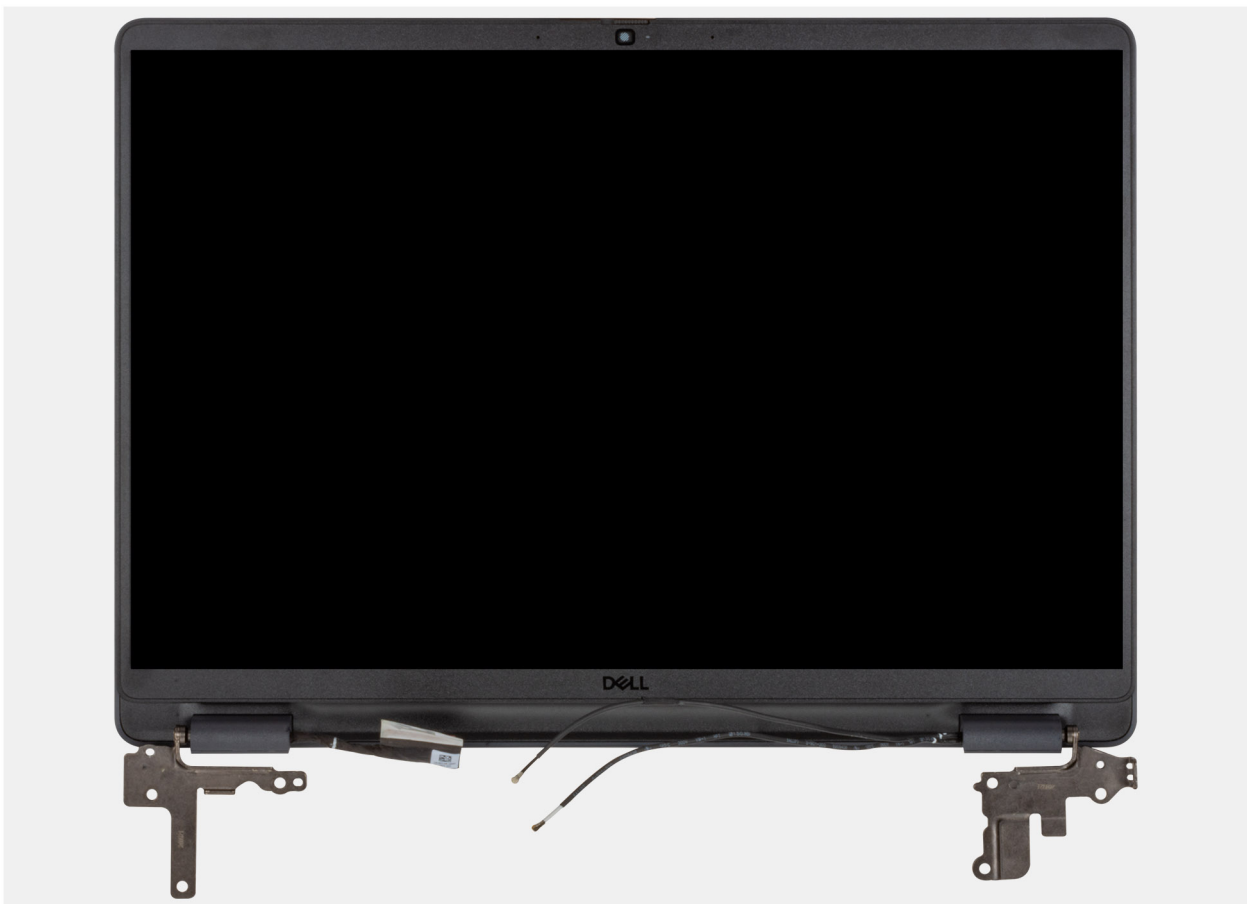
Figure 64. Removing the display assembly
