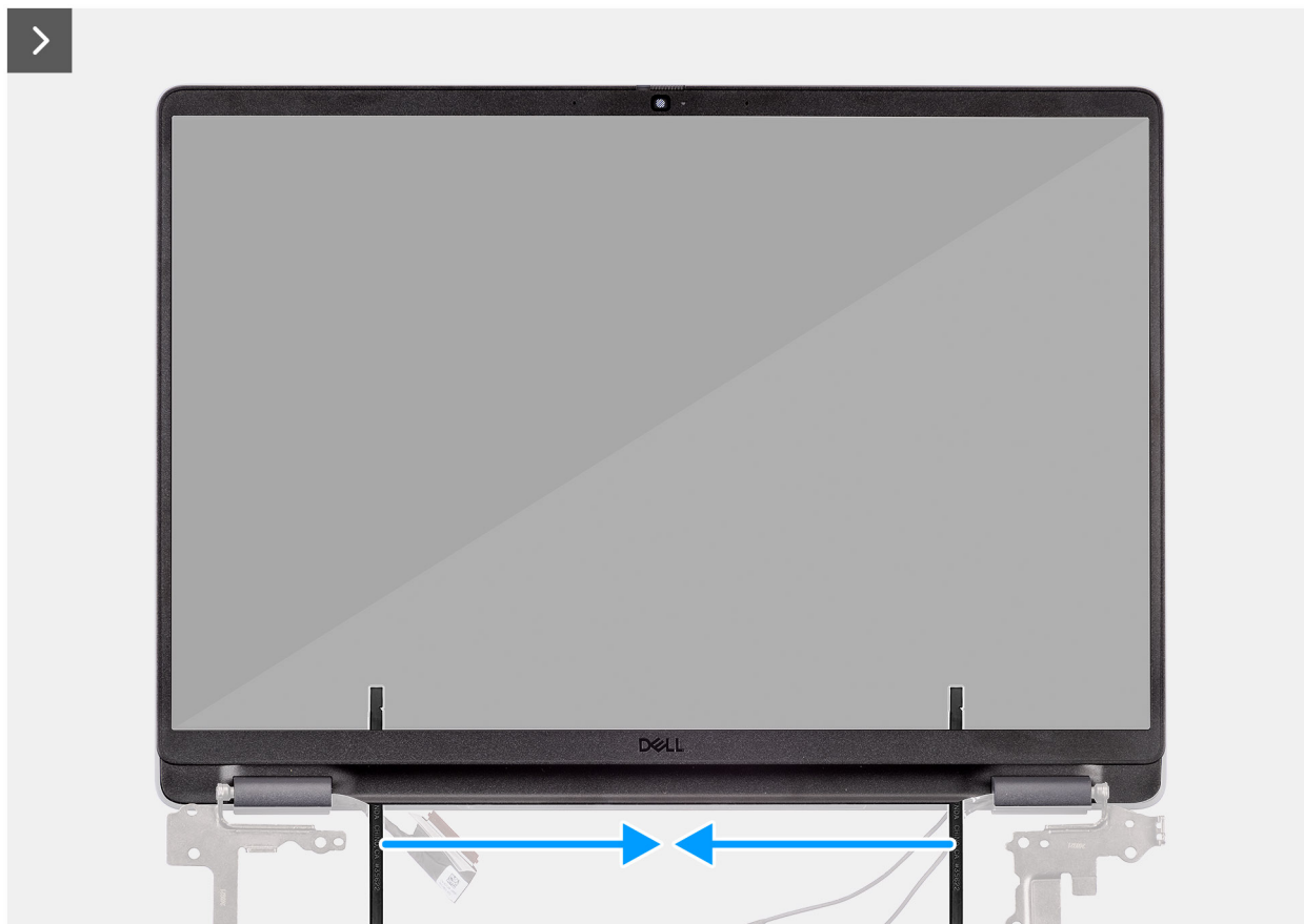
Figure 68. Removing the display bezel
