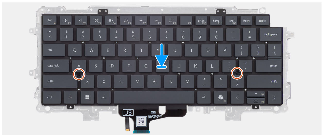
Figure 59. Installing the keyboard support plate
