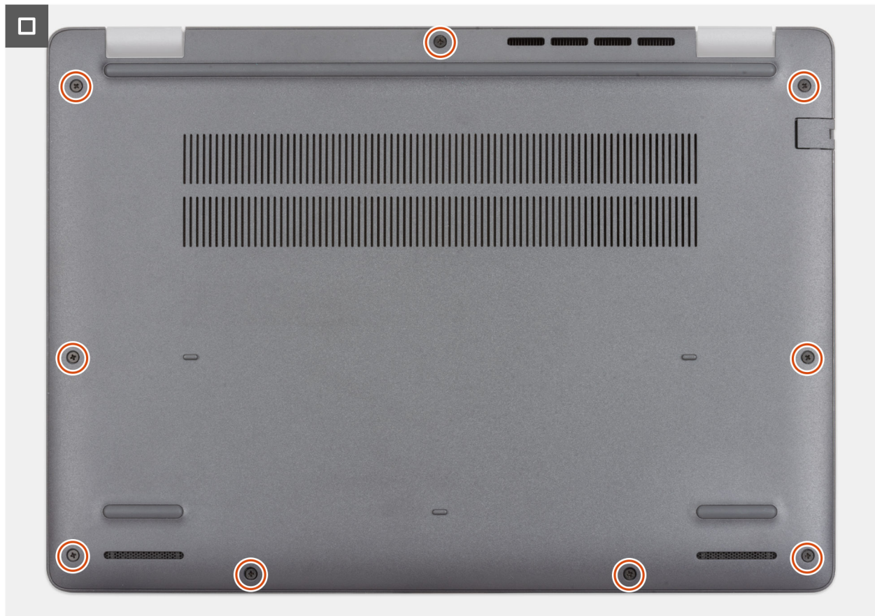
Figure 16. Installing the base cover
