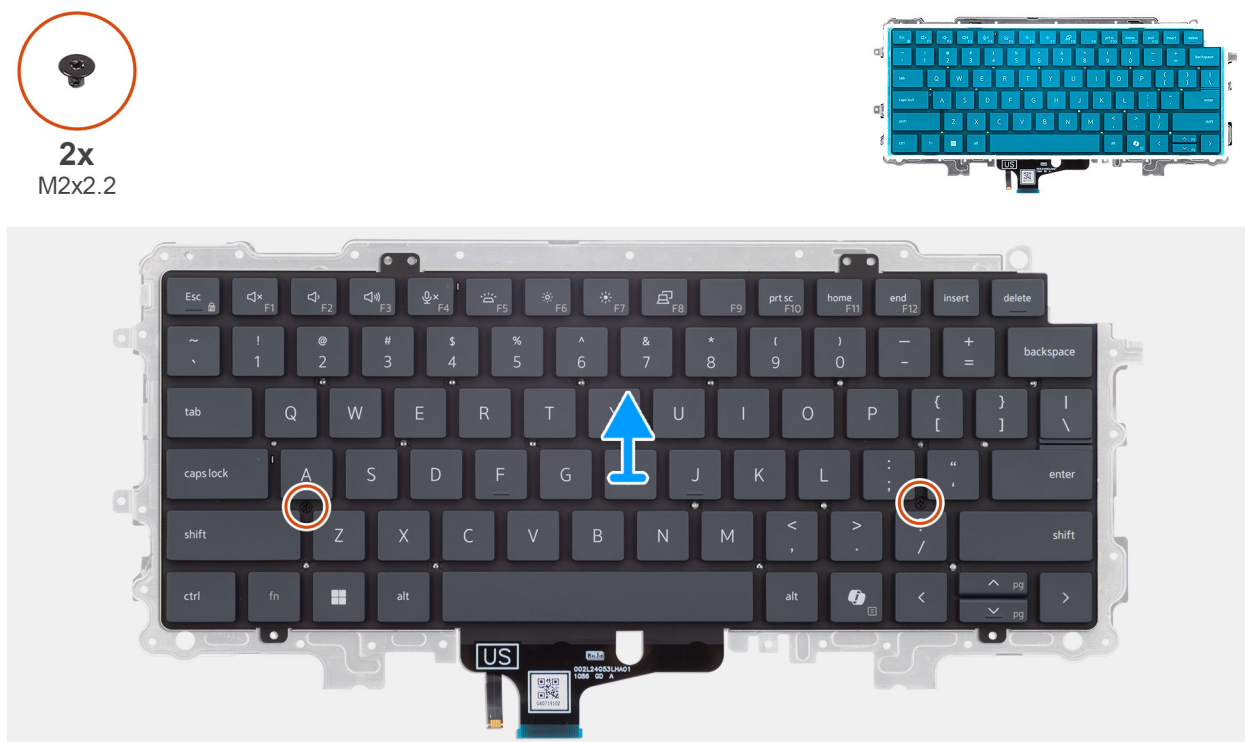
Figure 56. Removing the keyboard support plate
