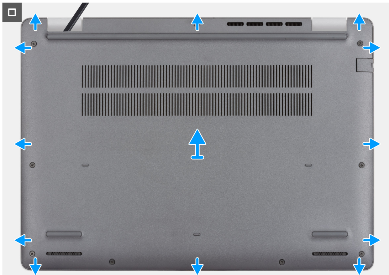
Figure 12. Removing the base cover
