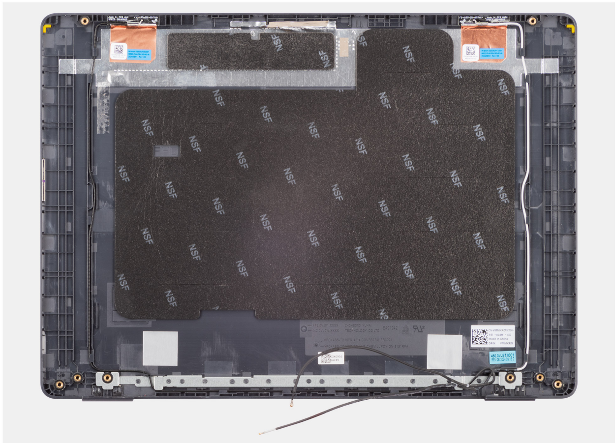
Figure 87. Installing the display back-cover assembly
