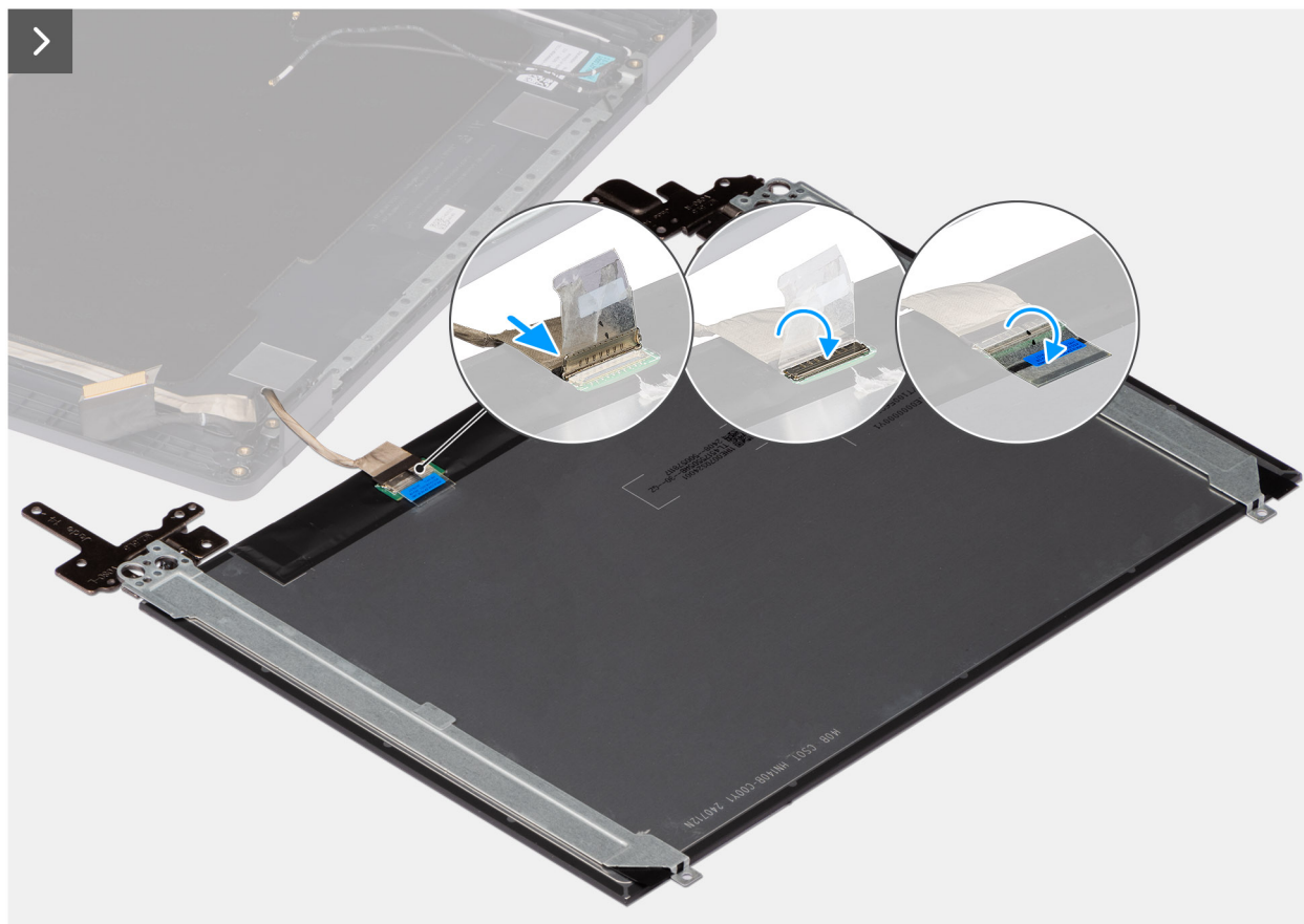
Figure 79. Installing the display-panel assembly
