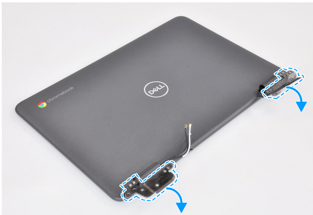
Figure 61. Display hinges are rotated to the unlock position
