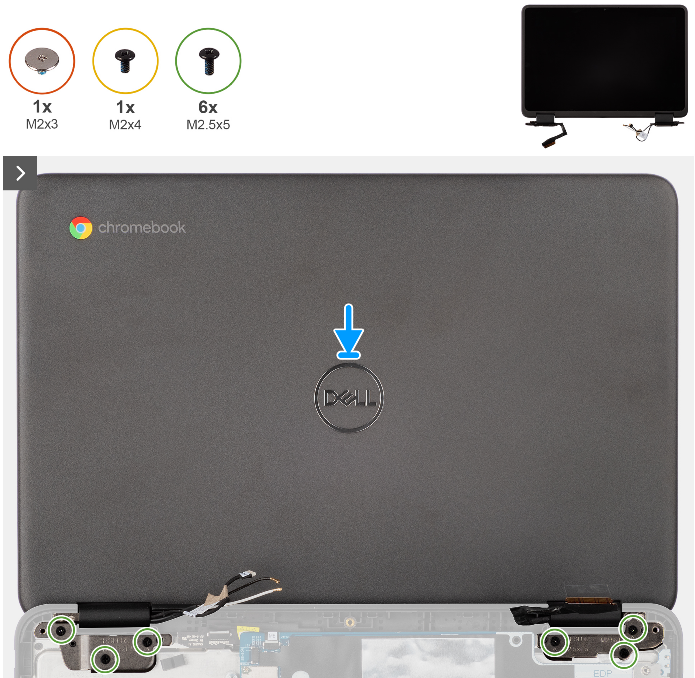
Figure 50. Installing the display assembly
