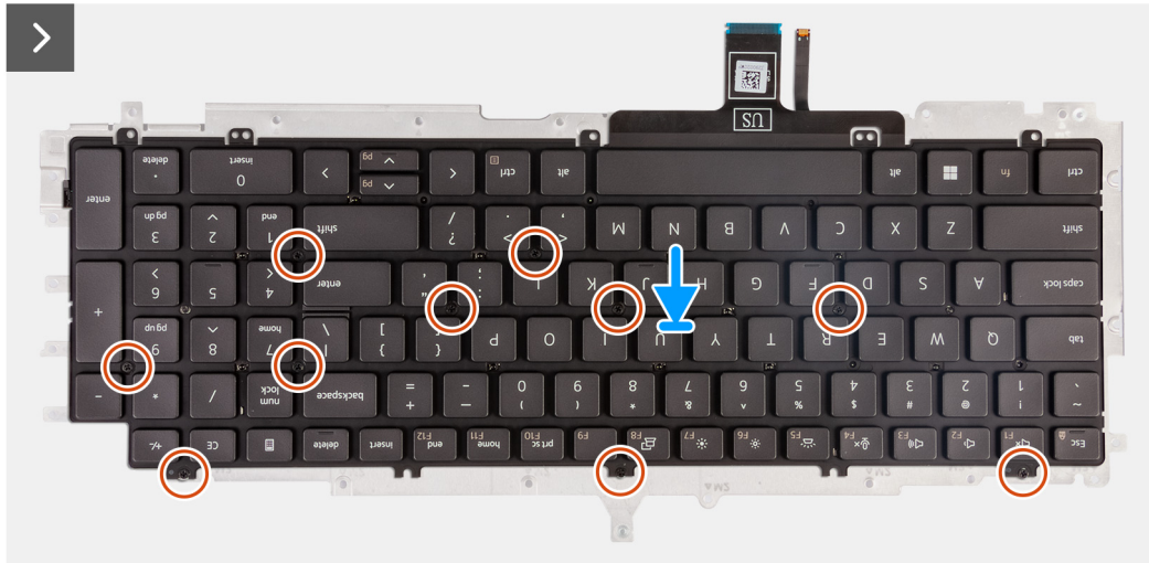
Figure 71. Installing the keyboard
