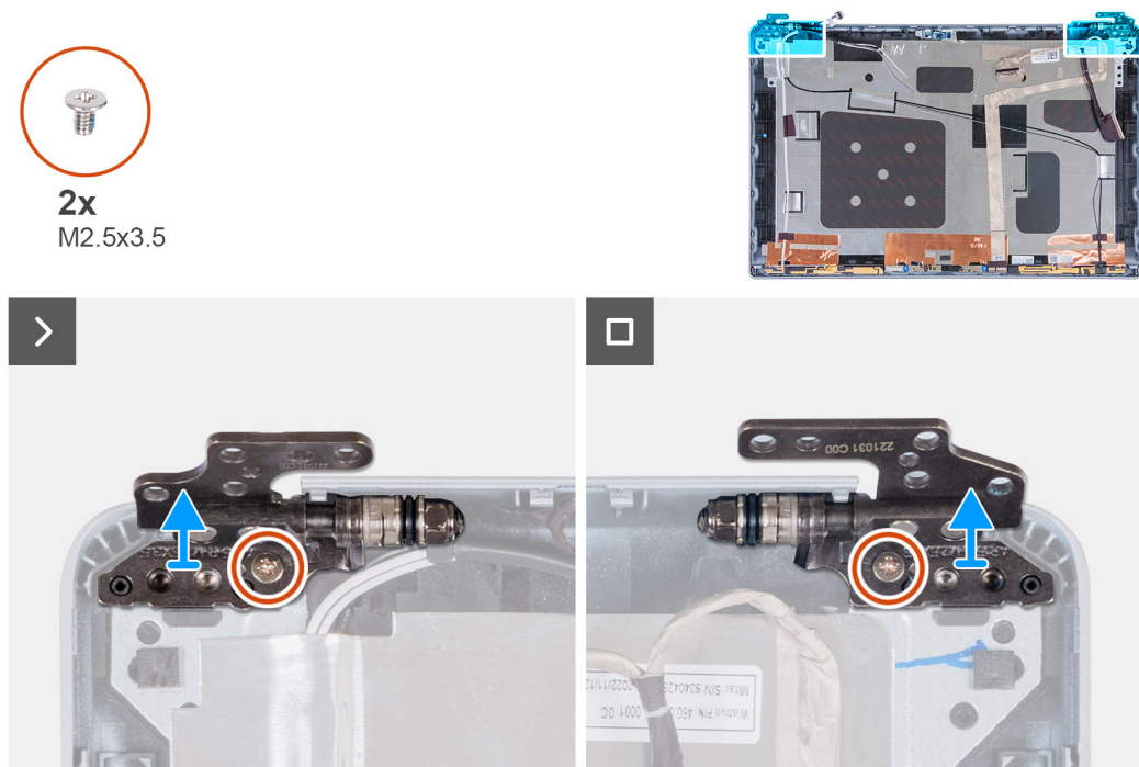
Figure 90. Removing the display hinges
