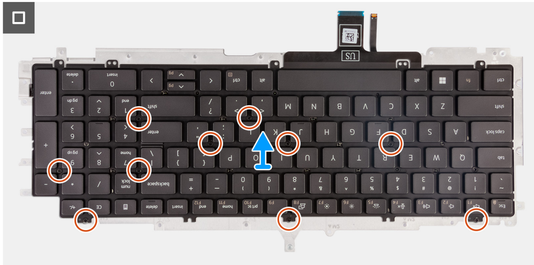
Figure 70. Removing the keyboard
