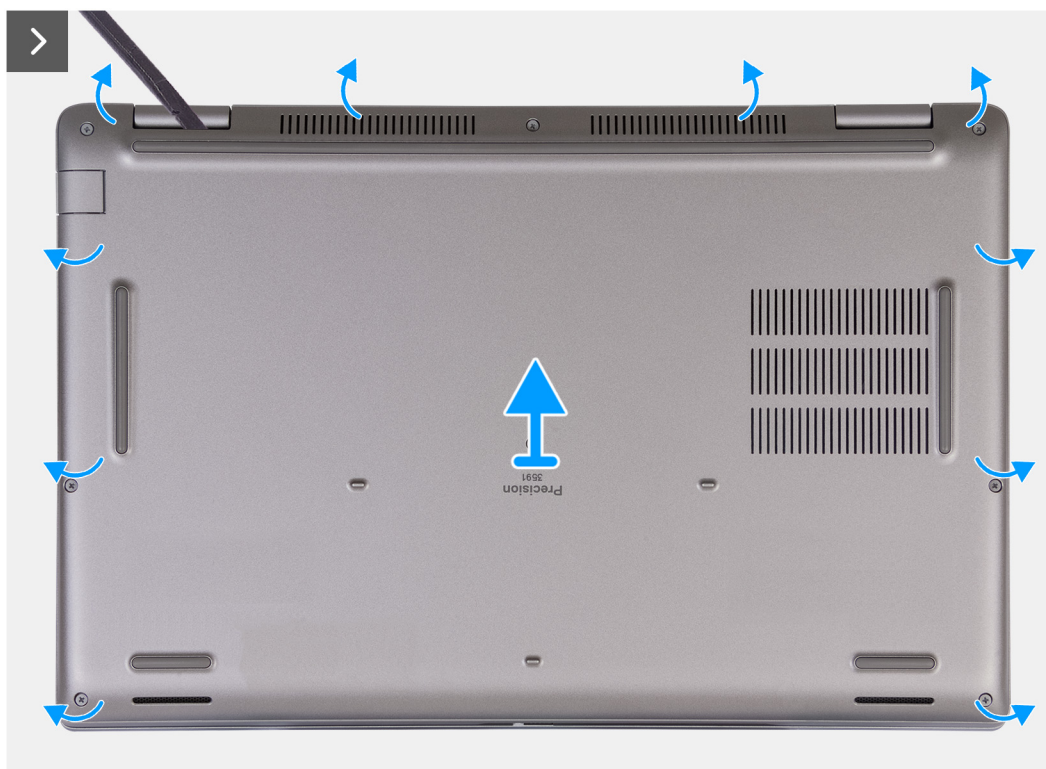
Figure 14. Removing the base cover
