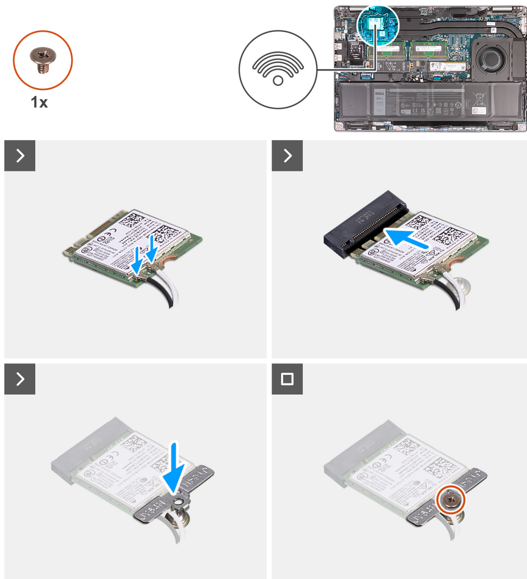
Figure 20. Installing the wireless card
