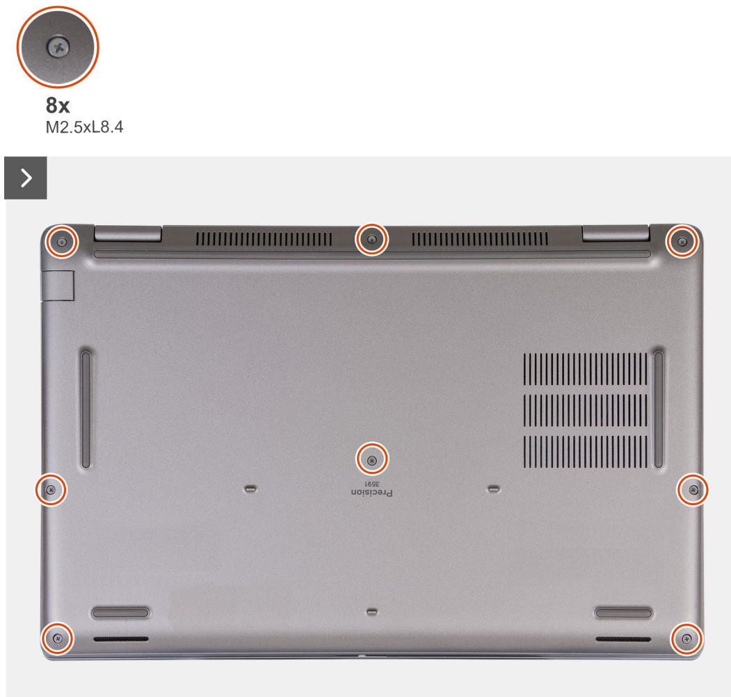
Figure 13. Loosen the captive screws
