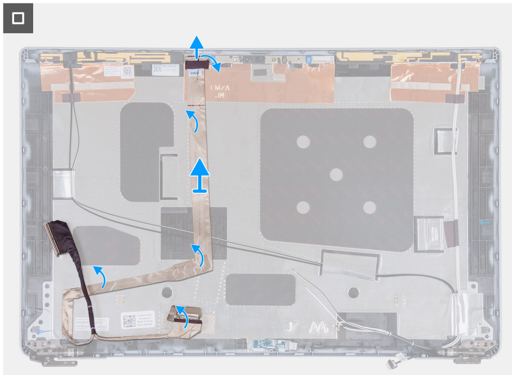
Figure 94. Removing the display cable
