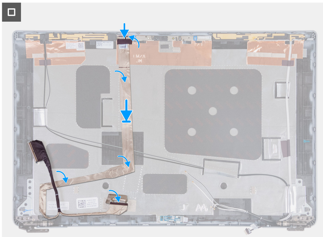
Figure 95. Installing the display cable
