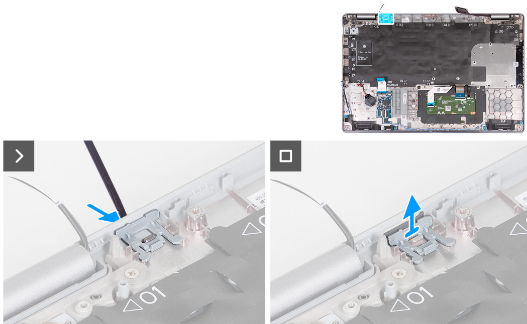
Figure 100. Removing the dummy SIM-card slot filler
