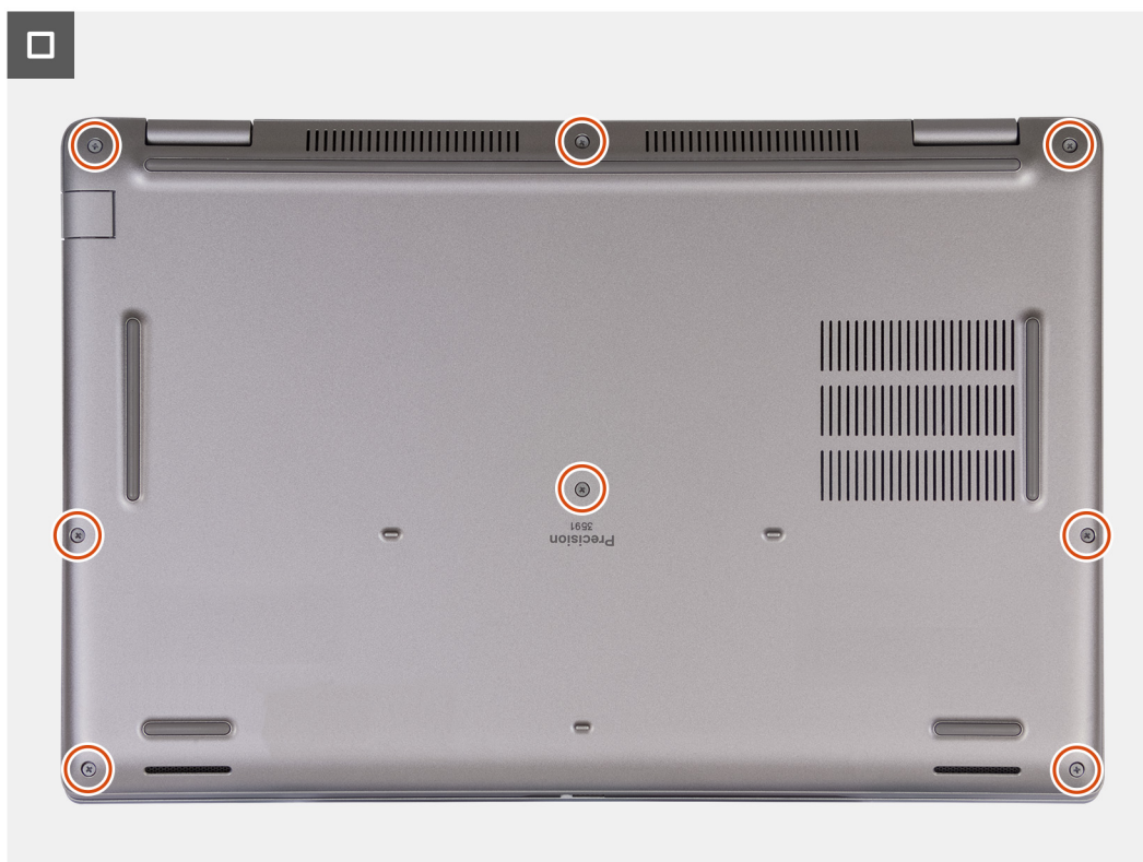
Figure 18. Tighten the captive screws
