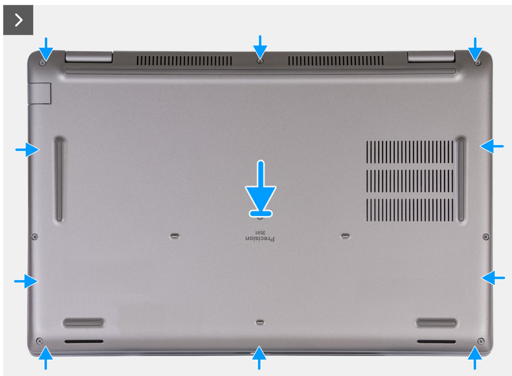
Figure 17. Installing the base cover
