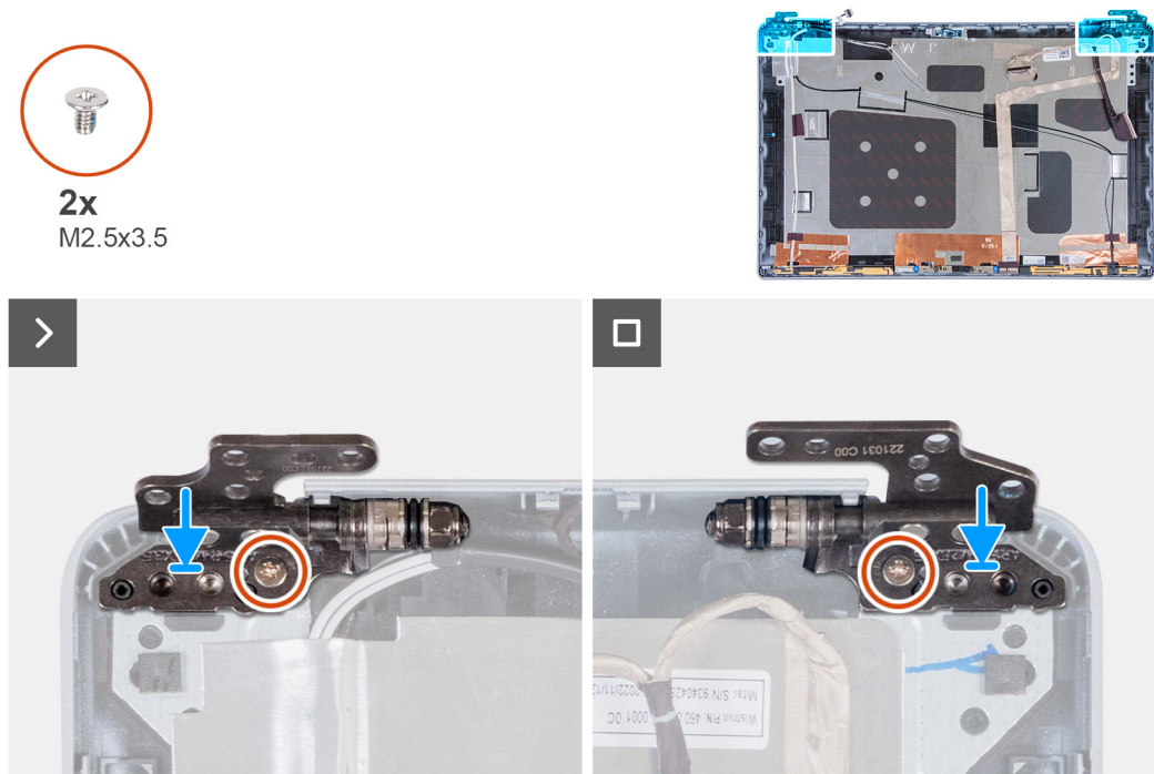
Figure 91. Installing the display hinges
