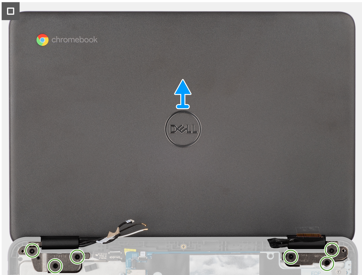
Figure 46. Removing the display assembly
