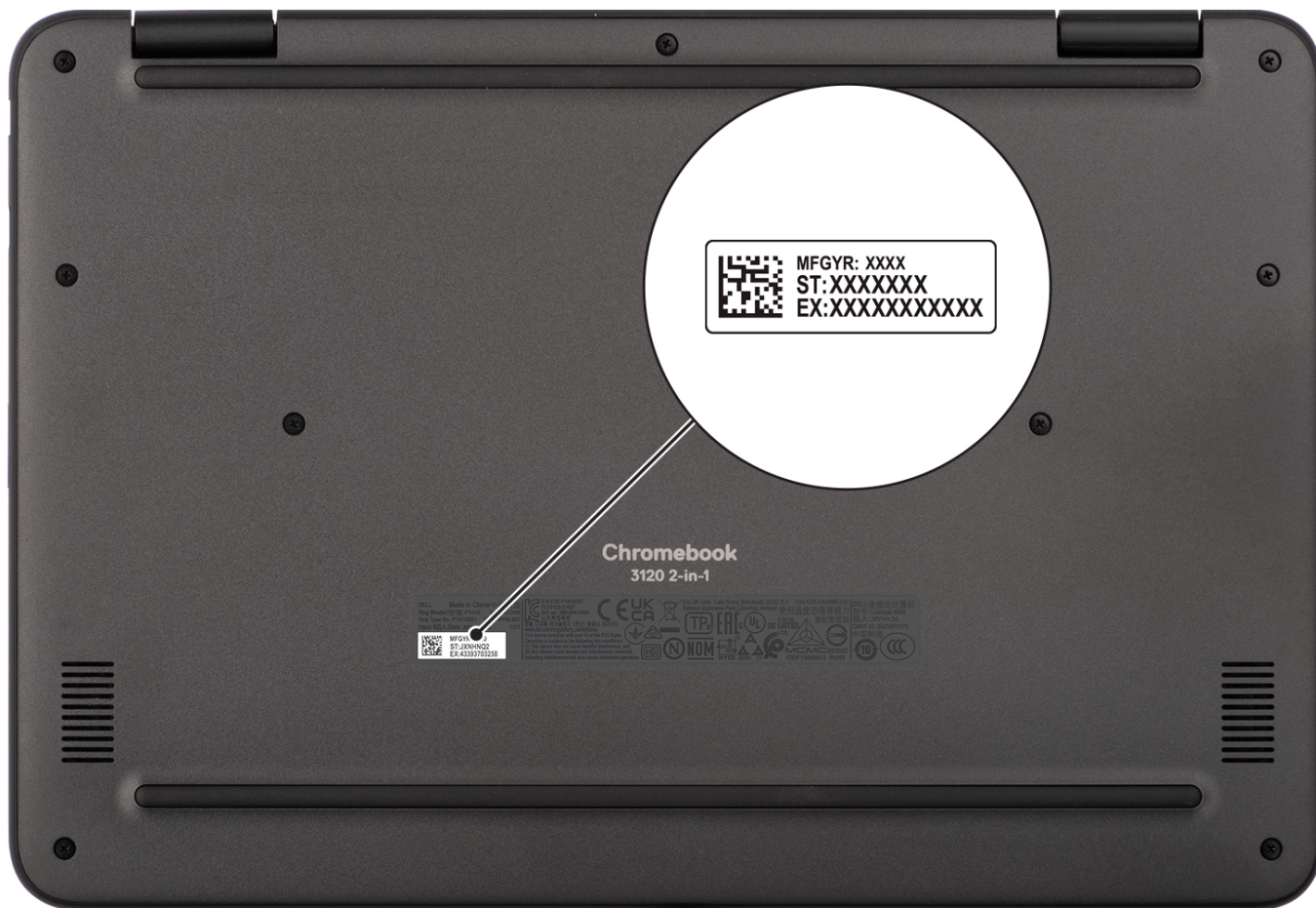
Figure 6. Service Tag location
