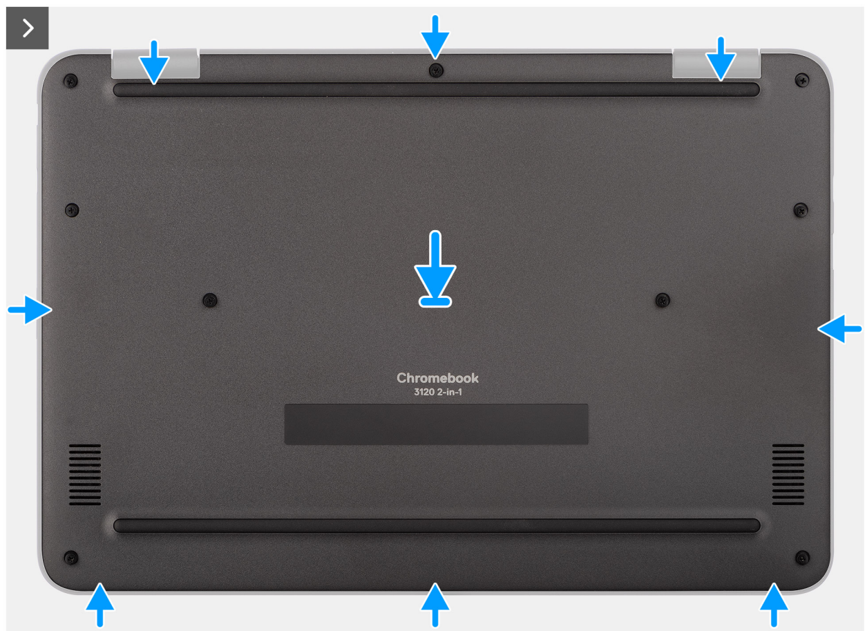
Figure 16. Installing the base cover
