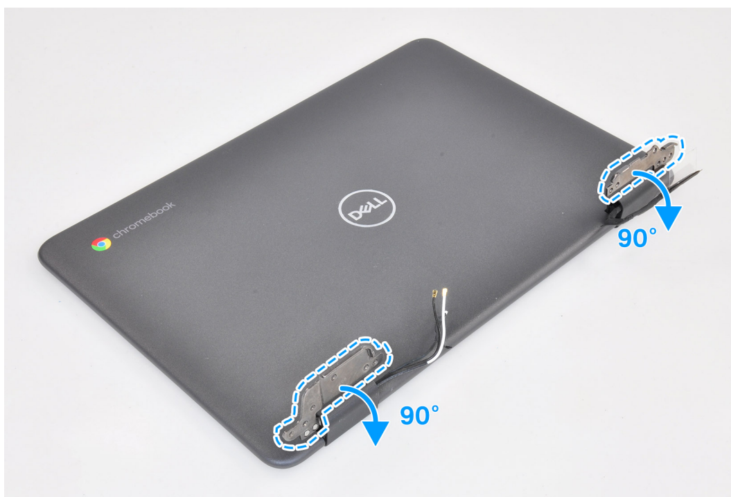
Figure 60. Display hinges and hinge cap angle
