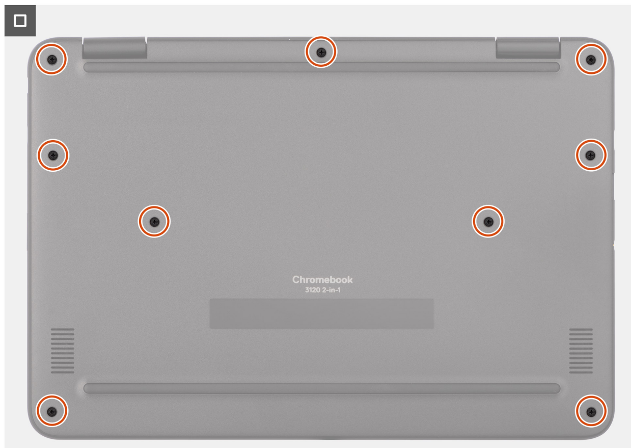
Figure 17. Installing the base cover
