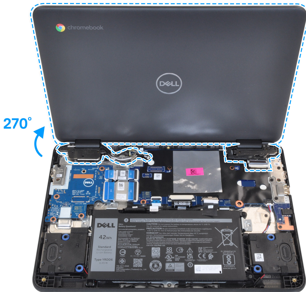
Figure 48. Open the system to 270 degrees
