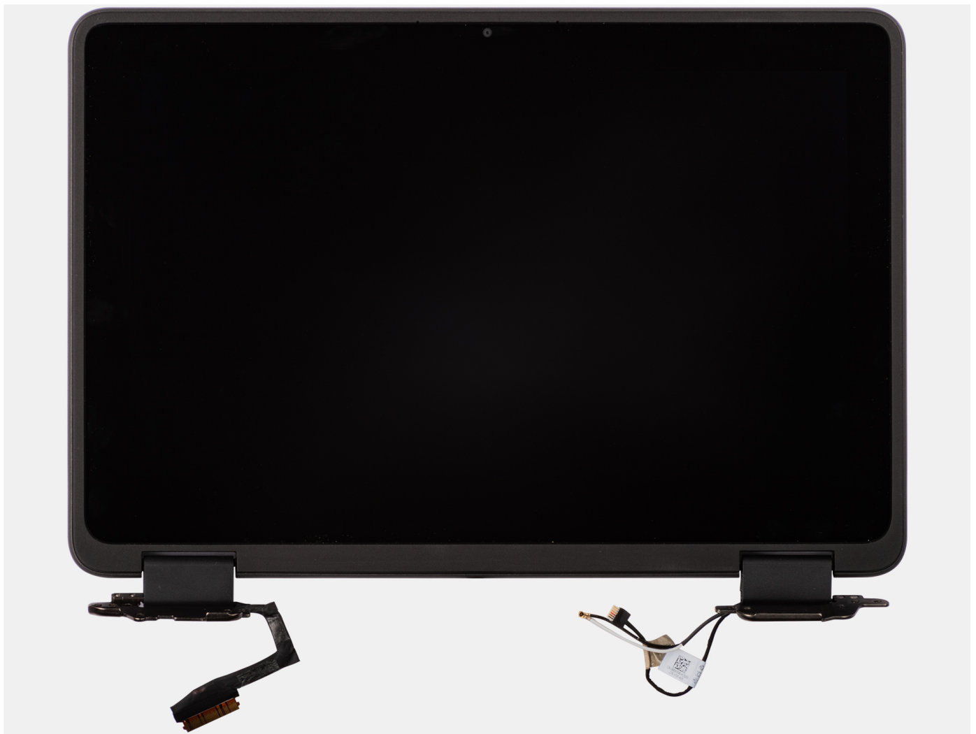
Figure 49. Installing the display assembly
