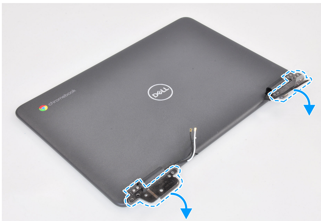
Figure 61. Display hinges are rotated to the unlock position
