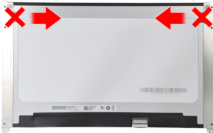
Figure 73. Stretch Release tape
