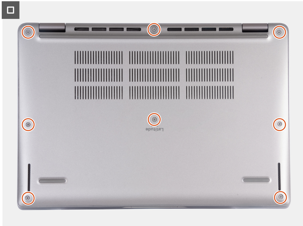
Figure 22. Tighten the eight captive screws to secure the base cover to the palm-rest assembly
