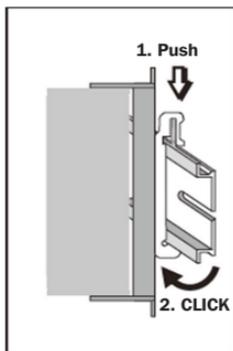
**Mounting the Switch    Removing the Switch**
