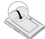
Place the back cover over the back of the device. Then press down along the edges to secure the cover.
