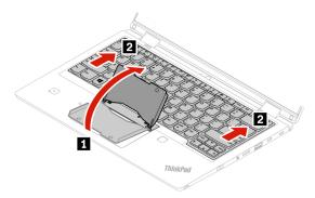
7. Pivot the keyboard slightly upward as shown by arrow **1**. Then turn the keyboard over as shown by arrow 2.
