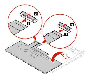
10. Insert the keyboard into the keyboard bezel as shown. Ensure that the front edge of the keyboard (the edge that is close to the display) is under the keyboard bezel.
