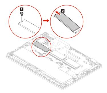
b. Slide the M.2 solid-state drive out of the Mylar film.
