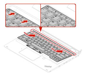
11. Slide the keyboard in the direction as shown by the arrows. Ensure that the latches are secured under the keyboard frame.
