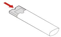
b. Insert the new M.2 solid-state drive to the drive slot. Then, pivot the drive downward and install the screw to secure the drive.
