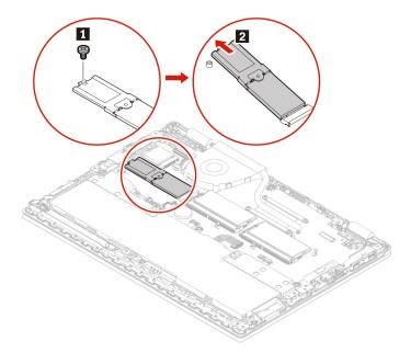
b. Turn the M.2 solid-state drive with the bracket over and remove the screw. Then, remove the M.2 solid-state drive from the bracket.
