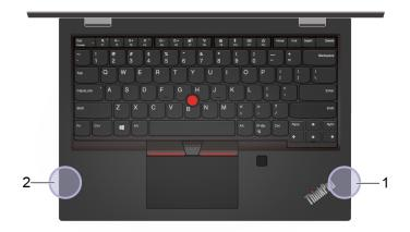
Wireless-LAN antenna (main) 2 Wireless-LAN antenna (auxiliary)
