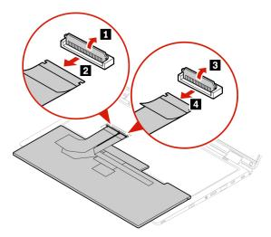
9. Attach the connectors and turn the keyboard over as shown.
