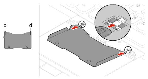
6. Pivot the tool in the direction as shown to release the keyboard ■. Push the keyboard in the direction as shown by arrows ■ to release the latches from the keyboard bezel.
