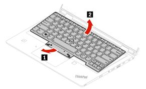
8. Put the keyboard on the palm rest as shown and detach the connectors. Then remove the keyboard.
