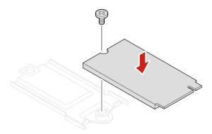
b. Turn the new M.2 solid-state drive with the bracket over. Insert the new M.2 solid-state drive to the drive slot. Then, pivot the bracket downward and install the screw to secure the bracket.
