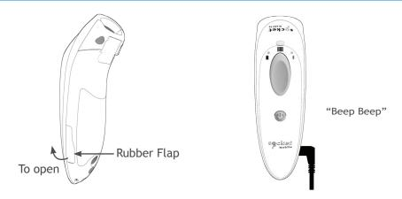
The scanner must be fully charged before first use. Please allow 6 hours uninterrupted charging for the *initial* battery charge. The scanner will stop charging once the battery is full (no overcharging occurs).
