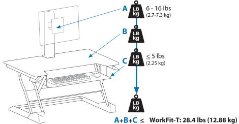
WorkFit-TL: 33.4 lbs (15.15 kg) WorkFit-TLE: 33.4 lbs (15.15 kg) WorkFit-TX: 33.4 lbs (15.15 kg) WorkFit-Corner: 28.4 lbs (12.88 kg)
