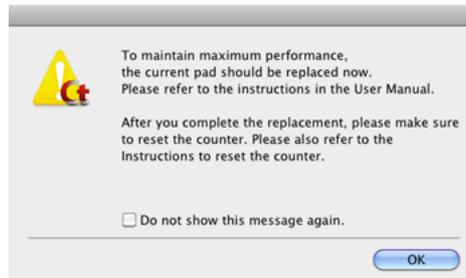
If this message begins to be displayed at startup, purchase an exchange roller kit and replace the worn parts with the consumable parts included in the kit (feed roller and retard roller). For details on the exchange roller kit, see "Exchange roller kit (product code: 5484B001)" on p.111.
