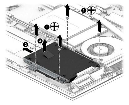
3. If it is necessary to disassemble the drive, remove the four Phillips M3.0×3.0 screws (1), and then remove the brackets from the drive (2).
