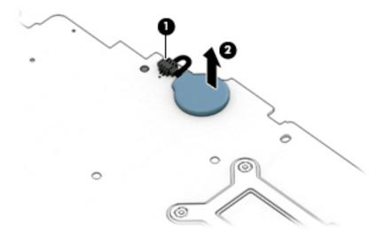
Reverse this procedure to install the RTC battery.
