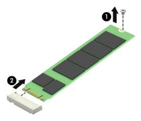
Reverse this procedure to install the Optane memory module.
