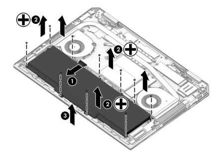
Reverse this procedure to install the battery.
