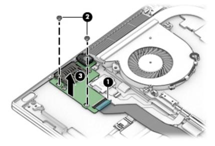
Reverse this procedure to install the card reader/audio board.
