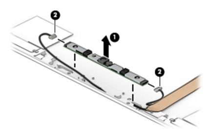
The camera module is available using spare part number L30660-001 for IR cameras.
