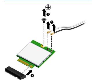
**NOTE:** WLAN modules are designed with a notch to prevent incorrect insertion.
