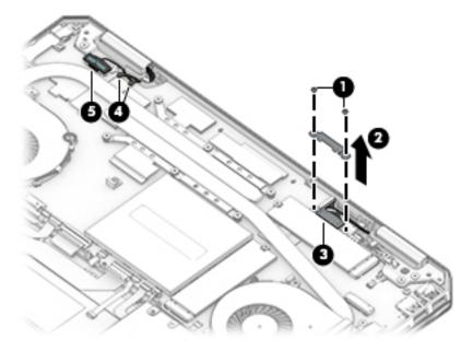
5. Remove the five Phillips M2.5×4.5 screws (1) that secure the display to the computer.
