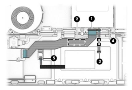
6. Remove the six Phillips M2.0×2.0 screws (1) that secure the TouchPad to the top cover.
