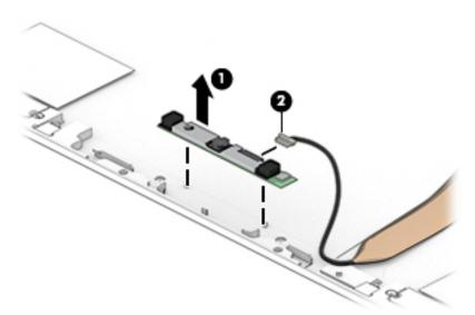
The camera module is available using spare part number L28470-001 for HD cameras.
