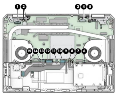
4. Remove the two Phillips M2.0×4.0 screws (2) from each fan.
