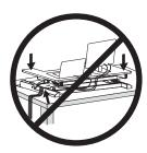
To avoid the potential to pinch cables it is important to follow the cable routing instructions in this manual. Failure to follow these instructions may result in equipment damage or personal injury.
