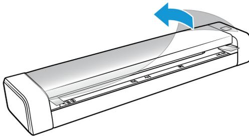
3. Place your thumbs on either side of the paper feed slot, underneath the lid of the scanner. Hold the scanner sides firmly and pull the scanner lid up to release it from the body of the scanner.
