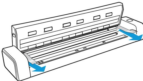
5. Gently close the scanner lid. Press down on both sides of the lid until you hear a click as the arms lock the scanner lid in place.
