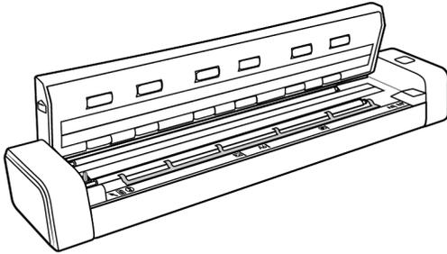
1. Place your thumbs on either side of the paper feed slot, underneath the lid of the scanner. Hold the scanner sides firmly and pull the scanner lid up to release it from the body of the scanner.
