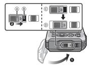
Do not open or close the side door in places with sand and dust, close to water, or with wet hands. Sand or dust adhering may cause water leaks.
