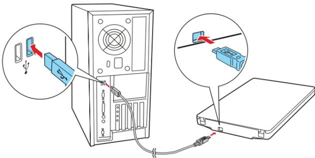
When the scanner is connected to the computer, it will automatically turn on. To turn the scanner off, disconnect the USB cable.
