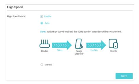
• Select the Manual mode and choose to transmit 2.4GHz band or 5GHz band only.
