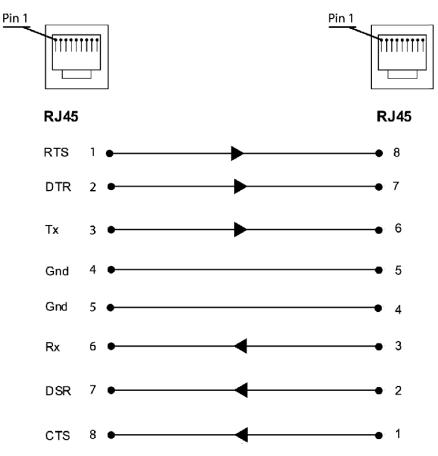
Figure E-5 RJ45 to RJ45 Adapter for Netra/Sun/Cisco and SLP (PNs 200.2225 and ADP010104-01)
