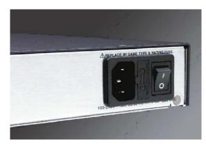
Figure 3-4 AC Power Input and Power Switch (SLCxxxx2N)
