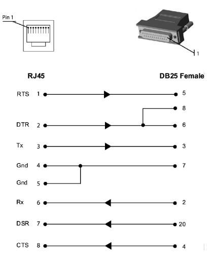
Figure E-2 RJ45 Receptacle to DB25F DCE Adapter for the SLC Console Manager (PN 200.2067A)
