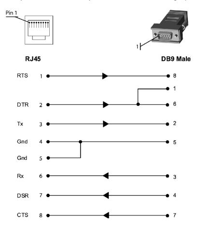
Figure E-3 RJ45 Receptacle to DB9M DCE Adapter for the SLC Console Manager (PN 200.2069A)
