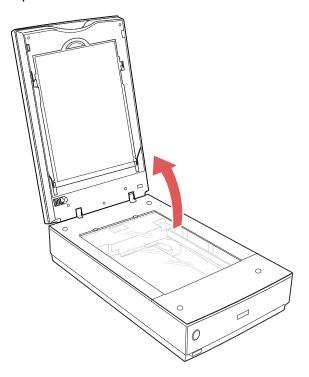
2. Make sure the document mat is installed inside the scanner cover.
