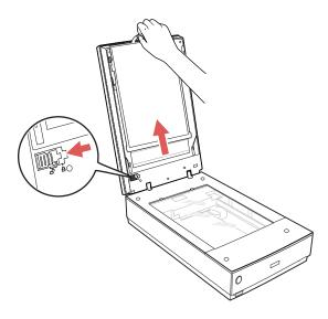
4. Clean the transparency unit window and the scanner glass before placing your film or slides.
