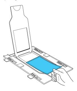
**Note:** You may need to trim the edges of the film so that it sits properly in the film holder without bending or warping. Do not cover any of the small holes in the holder.
