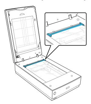
4. Place the film in the film area guide with the shiny side facing down. Make sure the entire image frame is positioned in the film holder opening.
