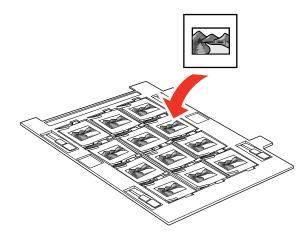
**Note:** The images and any wording on the slides should appear backward; the top of the images should face the open end of the slide holder. Do not cover any of the small holes in the film holder.
