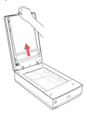
8. Lift the fluid mount tray off the guide and place it on the scanner. Orient it so the narrow window of the tray is toward the back of the scanner. Do not block the window.
