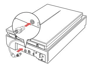
Note: Always turn off the scanner before connecting or disconnecting the cover cable.
