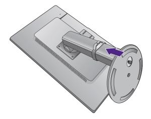
Rotate the turntable on the bottom of the monitor base until you see the thumbscrew (1).
