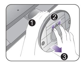
If the screen size is 27 inches, follow the illustration on the right to detach the monitor base. Release the thumbscrew on the bottom of the monitor base and detach the monitor base as illustrated.
