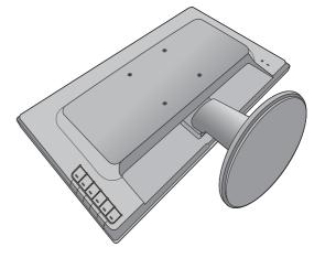
Insert a pointed object such as a screwdriver to the hole above the monitor stand arm, and then push the screwdriver against the release button inside the hole. Then pull the monitor stand backward away from the monitor.
