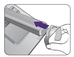
Orient and align the stand base socket with the end of the stand arm, then push them together.
