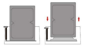
**Note:** We recommend ensuring the docking station is powered off before any drive is physically inserted or removed from the docking station. If two drives are docked simultaneously, and one drive is removed while the docking station is still powered on the other drive will momentarily disconnect from your computer which could cause drive damage or loss of data if other drive is still mounted.
