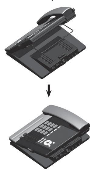
5. Install the wall mount bracket to the console as shown below. Insert the upper tabs of the mounting bracket into the upper slots at the back of the console. Press the lower tabs of the mounting bracket into the lower slots at the back of the console until they lock into place.
