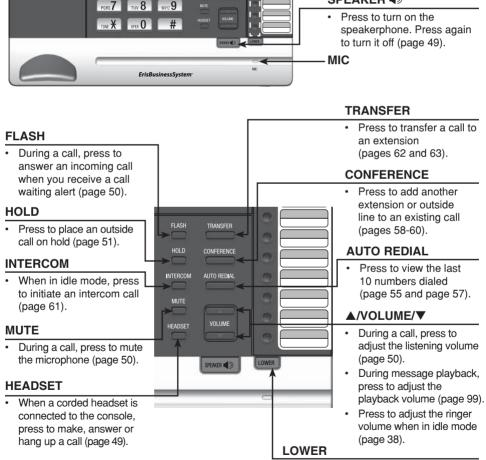
When assigning or dialing a one-touch number, press to switch to the lower location (the second 16 locations) of a one-touch key (pages 64-67).
