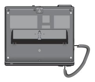
6. Connect the telephone line cords, Ethernet cable (if necessary) and power adapter as shown below.
