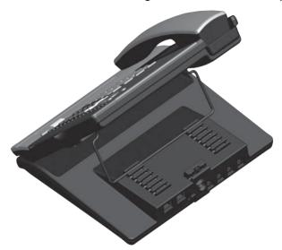
4. Connect the telephone lines, Ethernet cable (if necessary) and power adapter.
