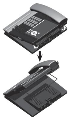
3. Snap the kickstand into the desired grooves until it locks into place.
