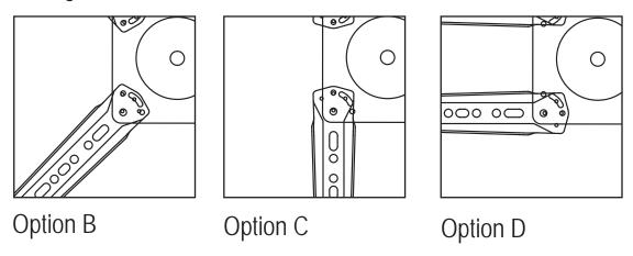
Rotate VESA plate to access mounting holes.
