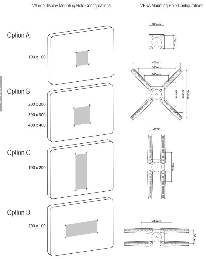
6 Option A: Attach TV/large display to the Glide LD using fasteners determined in step 4 and spacers if needed
