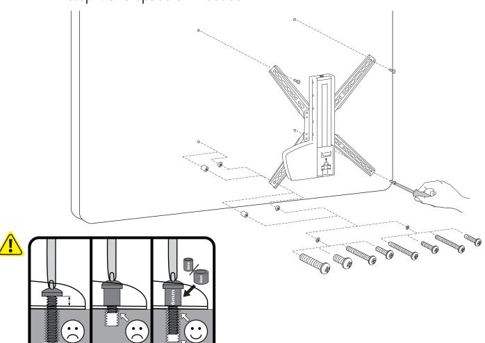
7 Mount the Glide LD (with attached TV/large display) to extension bracket on wall.
