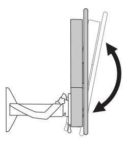
To change tilt angle, loosen knob, adjust and tighten knob.
