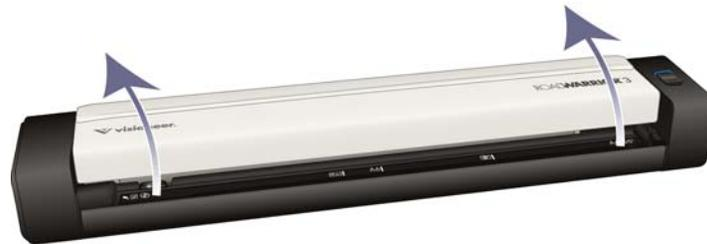
2. Hold the scanner sides firmly and pull the scanner top up to release it from the body of the scanner. Use both hands to open the scanner, the top is held down with locking arms on both sides of the paper feed slot. If you open only one side, you may warp the scanner top.
