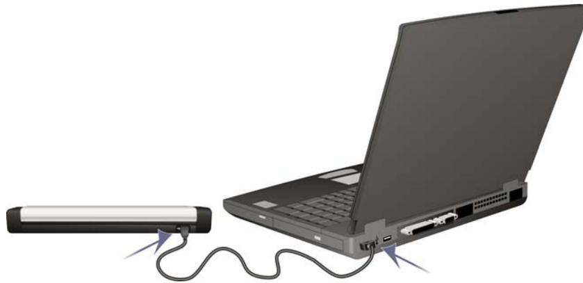
**NOTE:** If the plug does not attach easily, make sure that you are plugging it in correctly. Do not force the plug into either connection.
