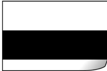
**Warning:** do *not* attempt to calibrate the scanner with any other type of document (i.e. white paper or a copy of the calibration page). The calibration routine will fail and indicate the failed calibration by flashing a red LED on the scanner. A calibration page was included with your scanner, if you do not have one available, you can order a replacement from the Parts & Accessories page for your scanner at [www.visioneer.com](http://www.visioneer.com).
