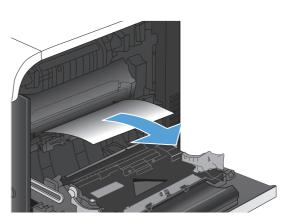
7. Look for paper in the Tray 2 roller area. Push up on the two green tabs to release the jamaccess door. Remove any jammed paper, and close the door.
