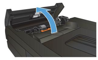
2. Use a moist, lint-free cloth to wipe both pickup rollers and the separation pad to remove dirt.
