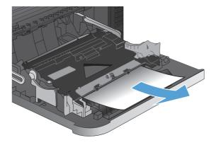
4. Lift the paper-feed cover on the inside of the right door. If jammed paper is present, gently pull the paper straight out to remove it.
