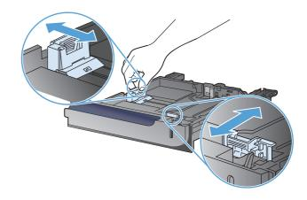
3. Load paper into the tray face-up. Check the paper to verify the guides lightly touch the stack, but do not bend it.
