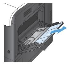
Fold out the tray extension to support the paper and open the side guides.
