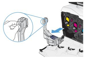
3. Place the attached blue cap over the blue opening at the top of the unit.
