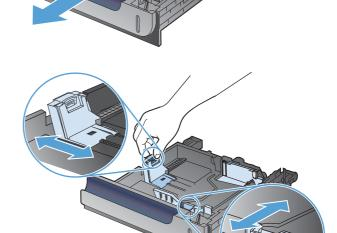
Load paper into the tray face-up. Check the paper to verify the guides lightly touch the stack, but do not bend it.
