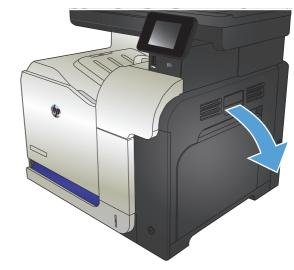
3. If paper is visible inside the right door, gently pull the trailing edge to remove it.
