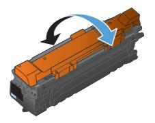
5. Remove the plastic shield from the toner cartridge.
