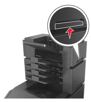
• If the printer does not have a caster base, then remove the optional trays.
