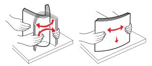
• Hold transparencies by the edges. Straighten the edges on a level surface.
