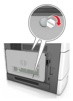
7 Reattach the controller board access cover.
