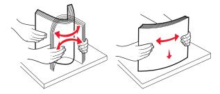
**4** Load the paper stack with the printable side facedown.
