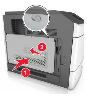
**6** Tighten the screws on the controller board shield.
