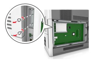
Remove the printer hard disk.
