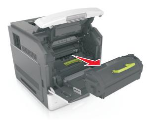
**3** Pull the imaging unit out of the printer using the handle.
