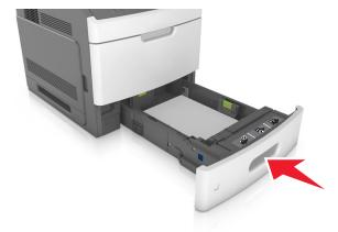
**8** From the printer control panel, set the paper size and type in the Paper menu to match the paper loaded in the tray.
