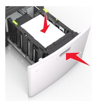
**6** From the printer control panel, set the size and type in the Paper menu to match the paper loaded in the tray. **Note:** Set the correct paper size and type to avoid paper jams and print quality problems.
