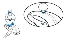
2 Choose the size and style of eartip that fits most comfortably. Align eartip tabs with notches in headset. Push in firmly and twist COUNTER clockwise.
