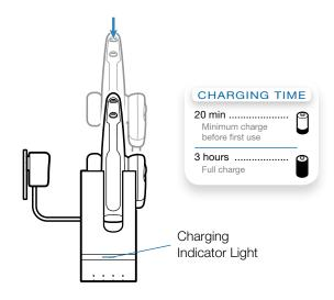
**NOTE** The USB charging cable can also be used to charge the headset. To successfully charge your headset with the USB cable the PC must be on and in an active state (not standby). The charging time will vary according to the number of other devices drawing power from the PC's USB port(s).
