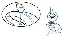
**NOTE** When installing a gel tip ensure the raised part of the eartip is pointed toward the curved section of the headset as shown.
