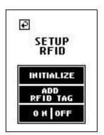
**Step 8:** Place the supplied RFID tag near the bottom right hand corner of the DL3 until you hear a "beep" tone.
