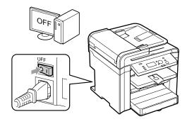
**2** Disconnect all cables and the power cord from the machine.
