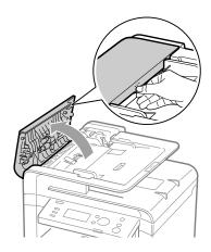
Clean the rollers (A) inside the feeder with a well wrung out cloth dampened with water, and then wipe the area with a soft, dry cloth.
