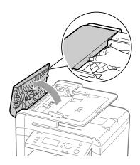
**3** Lift the lock release lever (A).
