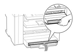
Pull out the output tray extension, and then lift the paper stopper.
