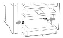
4 Pull out the output tray extension, and then lift the paper stopper.
