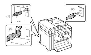
How to remove the cables and cord
