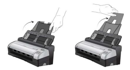
7. Pull the output tray away from the bottom of the Docking Station, then flip open the output tray extension.
