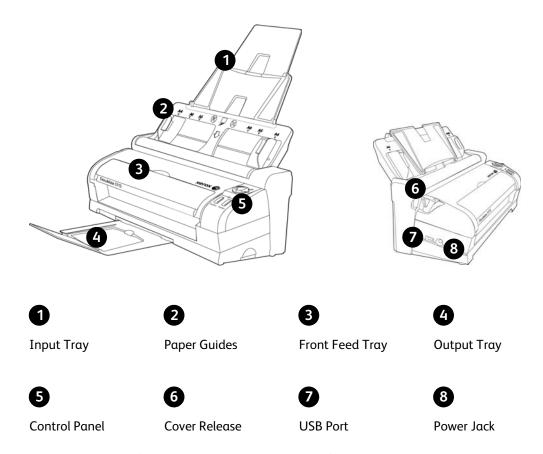
**Input Tray**—Holds a stack of documents in the scanner. Unfolds to support various paper lengths.
