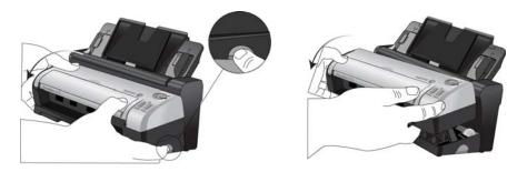
3. Remove the tape and foam strip from the docking station.
