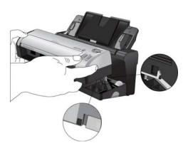
2. Tilt the scanner body into the Docking Station and press on the back of the scanner to lock it into the Docking Station.
