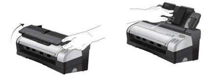
4. Pull the scanner cover release to open the scanner. Remove the foam strip from the inside of the scanner. Close the cover when you are done.
