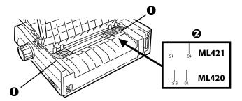
Note: The movement of the right tractor is limited to ensure that the paper covers the paper sensor.
