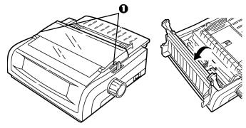
2 Remove the printhead shipping restraint.
