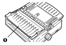
**3** Grasp the tabs and lift off the sheet guide.
