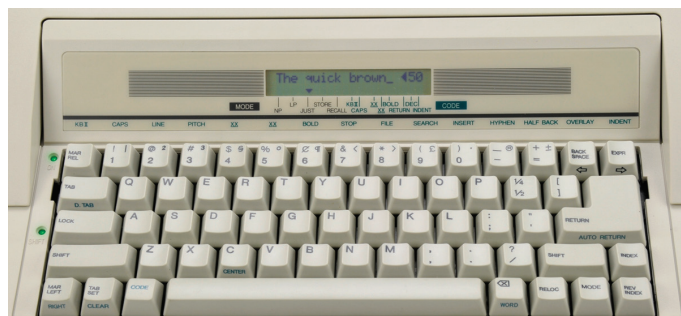
Full Size 45 Key and 17 Function Keyboard with 20 Character Liquid Crystal Display
