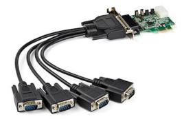
This PCI Express RS232 serial adapter card lets you add four RS232 (DB9) serial ports to your computer through a PCI Express (PCIe) slot. The 4 port PCIe serial card enables you to interact with serial devices, such as card readers, printers, PIN pads, and modems, at speeds of up to 921.6Kbps.
