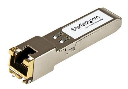
The AR-SFP-10G-T-ST is an Arista Networks SFP-1G-T compatible copper transceiver module that has been designed, programmed and tested to work with Arista Networks brand switches and routers. It delivers dependable 10 GbE connectivity over copper cable, for 100/1000/10000Base-TX compliant networks, with a maximum distance of up to 30 m (98.4 ft).
