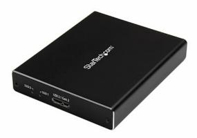
This dual-slot drive enclosure for mSATA and mSATA mini drives makes it easy to add ultra-fast, portable external storage to your USB-C or USB-A enabled laptop, tablet or desktop computer. The dual mSATA enclosure also provides RAID functionality for increased capacity, improved performance, or data redundancy.
