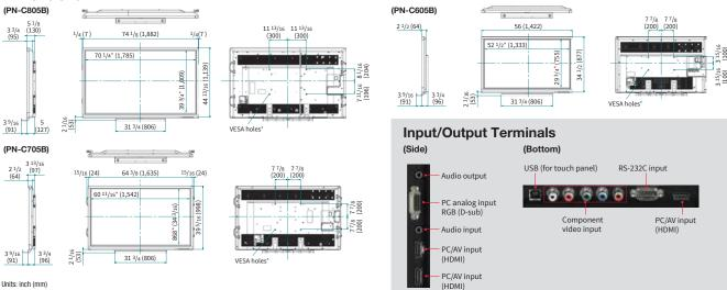
\* To use the VESA-standard mounting bracket, use M6 screws that are 8 to 10 mm plus the thickness of the bracket.
