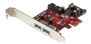
This PCI Express USB 3.2 Gen 1 card offers a cost-effective upgrade that lets you add four USB 3.2 Gen 1 ports to your computer through a PCIe slot. It offers two external ports plus two internal (IDC) USB 3.2 Gen 1 headers to help adapt your desktop or server to support a variety of USB 3.2 Gen 1 devices.
