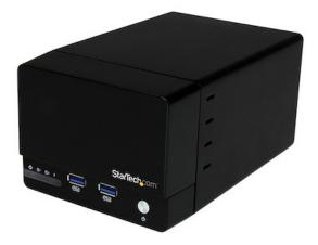
The S352BU33HR 2-Bay RAID Enclosure lets you build an external RAID array using two 3.5" SATA hard drives, and add it to your computer through USB 3.0.
