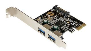
The PEXUSB3S23 2-Port PCI Express USB 3.2 Gen 1 Card lets you add two USB 3.2 Gen 1 ports to any PCI Express-enabled computer system. The USB card requires SATA power for functionality, and delivers 900mA of power per port to USB 3.2 Gen 1 bus-powered devices (500mA for USB 2.0) via your computers SATA power connector.
