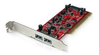
The PCIUSB3S22 2-Port PCI to USB 3.2 Gen 1 Card enables you to connect USB 3.2 Gen 1 peripherals to a PC through a legacy PCI host bus, which doubles the data transfer speeds when used with USB 3.2 Gen 1 peripherals than would be possible with a USB 2.0 host connection - up to 1.3 Gbps (PCI bus limit).
