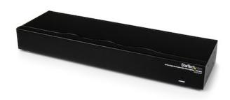
This high resolution VGA splitter offers a practical solution for high-res multi-screen presentations, allowing a VGA video signal to be broadcast from a computer to up to 16 VGA monitors simultaneously.
