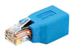
This is a technician's tool. The adapter converts a regular RJ45 cable into a Rollover cable. Used to connect a computer terminal to the console port on a router, it is a type of null modem cable. Also called a "Yost" cable. Copy should include that the device conforms to the "Yost Serial Device Wiring Standard"
