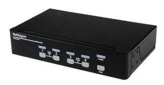
This 4 port DVI USB KVM Switch lets you control four USB enabled, DVI capable computers from a single USB keyboard and mouse peripheral set.
