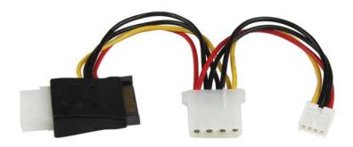
This LP4 to SATA Power Adapter Cable features an LP4 female connector as well as an SP4 female power connector and a SATA power connector, allowing you to connect an IDE hard drive as well as a floppy disk drive to a Serial ATA power connector provided by the computer power supply.
