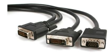
The DVIVGAYMM6 6-foot DVI-I (male) to DVI-D (male) and HD15 VGA (male) video splitter cable lets you connect a DVI-D monitor as well as a VGA monitor to a single DVI-I video card port.
