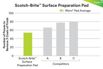
\*Pads worn via 25 passes over 3M™ Safety-Walk™ Slip-Resistant Treads 610 (swing machine)
